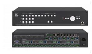
The VP-554X is a high-performance presentation scaler/switcher with 4 pairs of independent and scaled outputs. It includes multiple HDMI and HDBaseT inputs – supporting resolutions up to 4K – as well as a legacy VGA input, and each of the 4 outputs is mirrored on both HDMI and HDBT.
